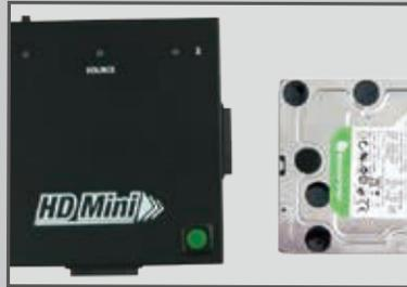
2. Plug in the source HDD and target HDD(s). The correspondent LED will be on if the HDD is connected well.
