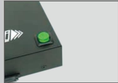
3. Press down the green button, the HD Mini will start duplication automatically and the LED(s) will keep flashing.
