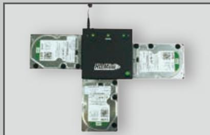
4. After copy is done, the green light will stop flashing and stay on with a warning sound to tell the finish of duplication. If there is error during the duplication, the green light will go off with two warning sound as signal.
